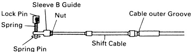
② Fitting of Remote Control Cable to Engine
